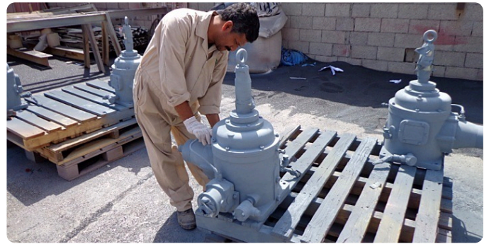
Epoxy coating of steel parts
